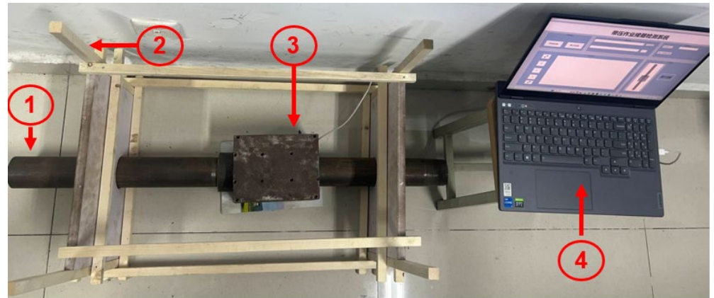
1-Measured pipe 2-Test rack 3-Pipe coupling detection device 4-Upper computer
