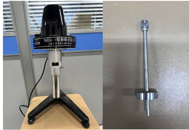
(a) NDJ-1 Rotational Viscometer (b) Rotor No. 2
