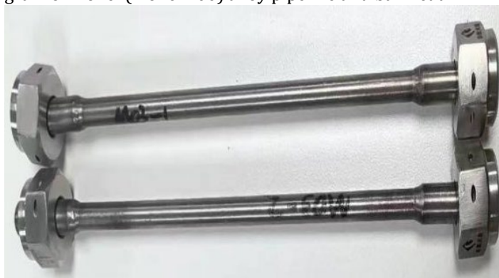
Figure 1. Welding of pipeline and ball head
