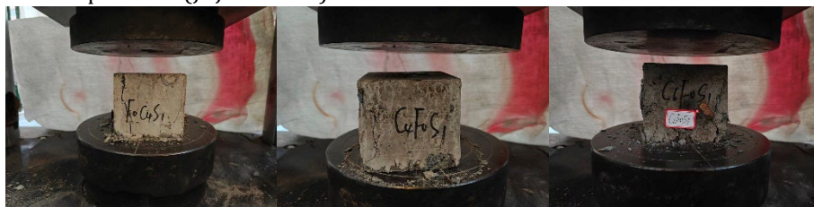
Figure 1. Failure Modes of Concrete
