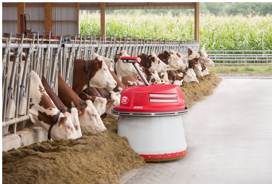
Figure 3. Intelligent Feeding Pusher Robot
