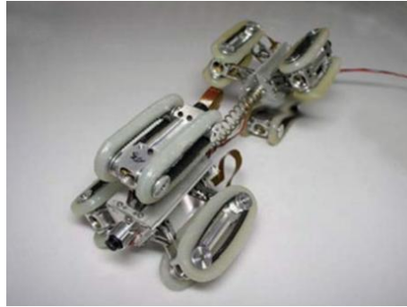
Figure 4. Tracked Pipeline Robot
