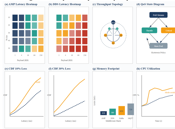
Figure 5. Adaptive middleware performance panel with eight subfigures. Panels (a) and (b) compare end to end latency heatmaps for the proposed AMP and default data distribution service across node cardinality and payload size. Panel (c) depicts message throughput as a radial topology graph. Panel (d) illustrates the quality of service state transition diagram. Panels (e) and (f) provide cumulative latency distributions under 10 percent and 30 percent packet loss. Panel (g) compares memory footprint across middleware stacks. Panel (h) shows central processing unit utilization during an adaptive mode transition event.
