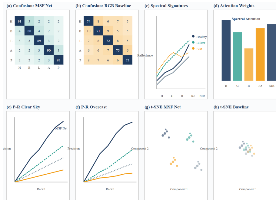
Figure 3. Comprehensive multispectral perception evaluation panel comprising eight subfigures. Panels (a) and (b) display normalized confusion matrices for the proposed MSF Net and the red green blue baseline respectively. Panel (c) illustrates mean reflectance signatures across five spectral bands for three representative classes. Panel (d) visualizes the learned spectral attention weights. Panels (e) and (f) present precision recall curves under clear sky and overcast illumination for four compared methods. Panels (g) and (h) show two dimensional t distributed stochastic neighbor embedding projections of latent feature spaces for the proposed and baseline networks.
