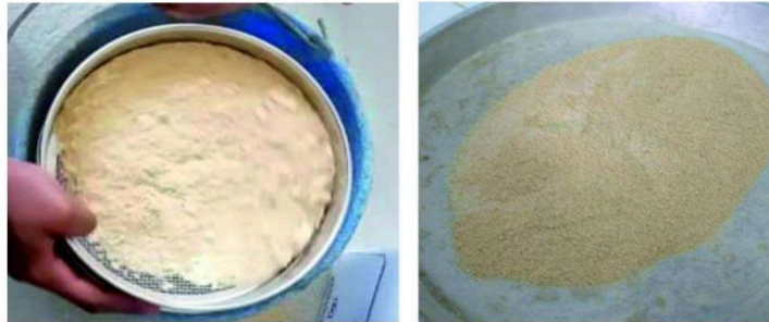
Figure 3.3. Sieving of the sawdust
