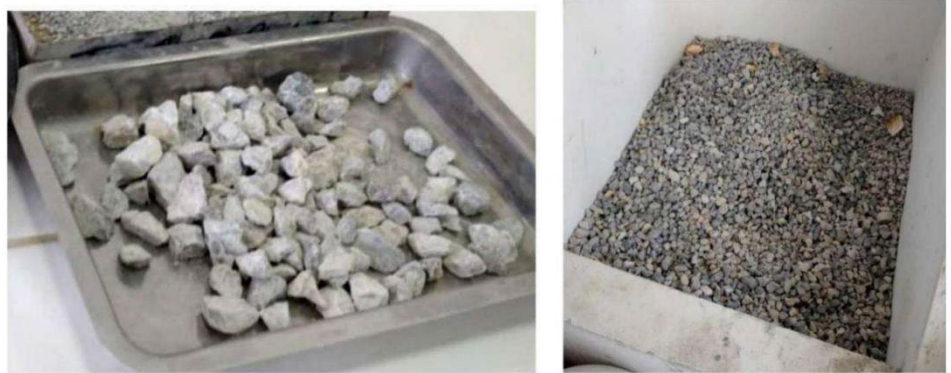
Figure 3.1. Sample of Coarse Aggregates Used (Size Range: 12.5 mm - 19 mm)
