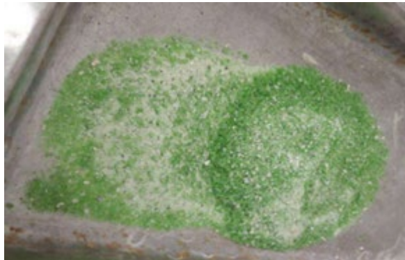
Figure 3.2. Sample of the glass powder used
