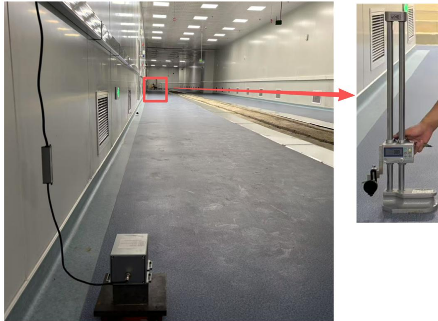
Figure 2. Schematic diagram of calibration process for static deflection indication error of deflection measuring instrument based on height capiler
