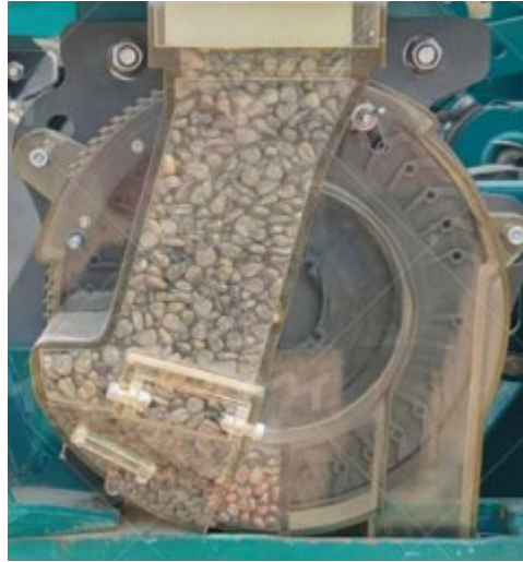
Figure 3. Air-suction seed meter
